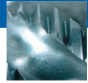
■ Cutting edge after 1.000 holes tapping
